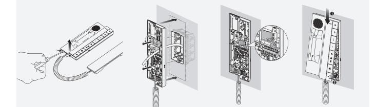
It can be surface mounted directly using wall plugs, using the Vimar flush mounting box for masonry walls or hollow walls, either round ø 60 mm or rectangular with 3 modules, or a British standard square mounting box.
